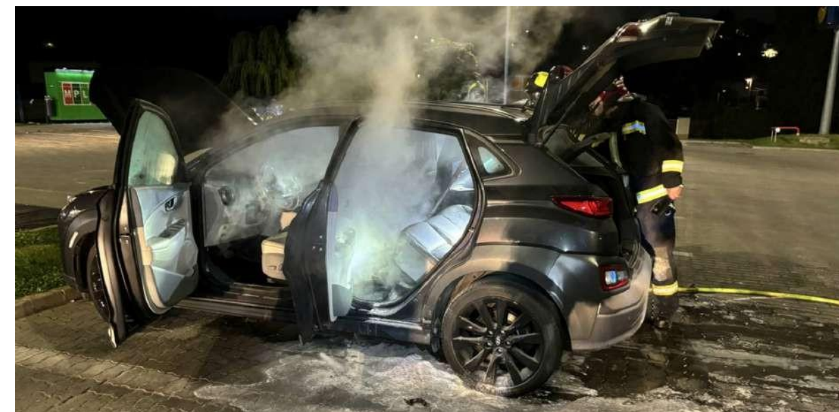
The white smoke coming from the electric vehicle indicates a damaged battery – Source: infostart.hu
